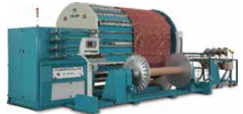
Sample Warper RI 601 (190 cm / 7-105 meter / 8 colours)
