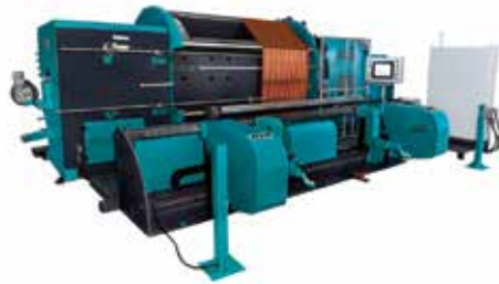
High Speed Automatic Sample Warper RI 6001 (220 cm / 27-500 meter / 16 colours)
